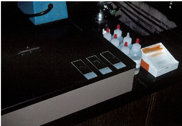
Figure 7.3 A Typical Slide Warmer Used to Speed Up the Drying of Slides.
